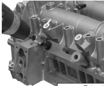
Extracting glow plug tube.
